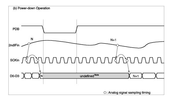
**Note** The output data is undefined from the start of the power-down operation to the 7.5th clock from the falling edge of the clock at which the power-down operation is cleared.
